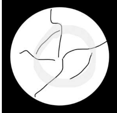
Figure 1.10: Schematic illustration of cracking in a UO 2 fuel pellet.
